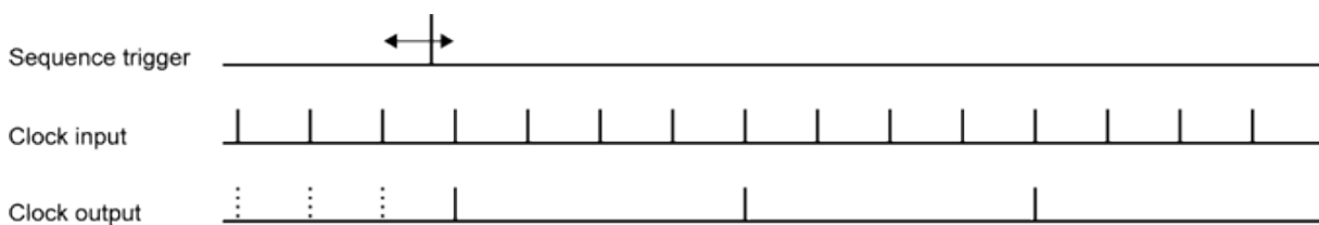
Beginning of an acquisition sequence for a value N of 4
