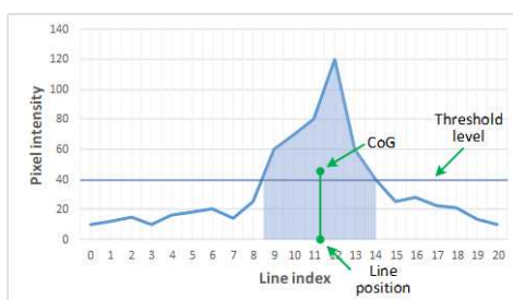
Center of gravity on a ROI profile
