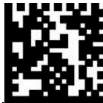
A data matrix showing mark growth
