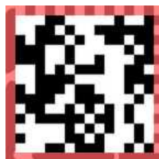
A data matrix showing finder pattern defects
