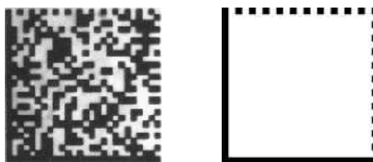
ECC 200, 26x26 cells data matrix code (left) and finder pattern (right)
