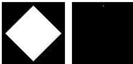
Source image (left) and top corner detected in the source image (white dot)
