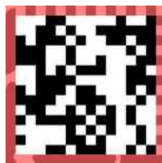
A data matrix showing finder pattern defects
