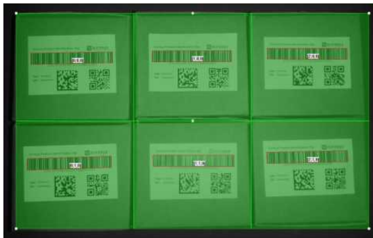
Reading of bar codes arranged in a grid
