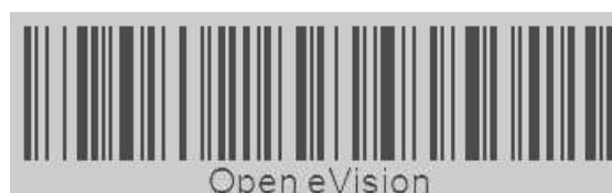
The bars and the spaces are too close on the gray scale
