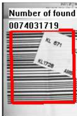
Occluded bar code (left) and a quiet zone that is too small at the top (right)
