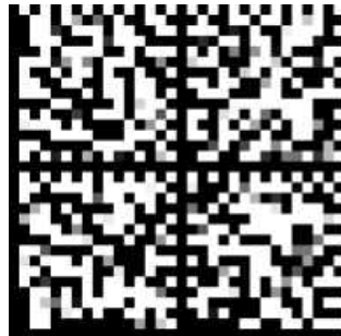
A data matrix with a low modulation grade
