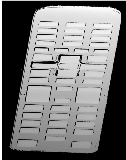
A depth map of the TV remote controller (the object is distorted and scaled while black pixels represent undefined regions, that is parts of the object that were not seen by the camera or lit by the laser)
