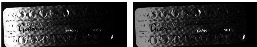
The object image: raw (left) and after correction with the flat image (right)
