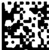
A data matrix showing cell defects
