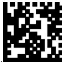
A data matrix showing mark growth
