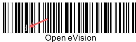
There is a light defect in the bar
