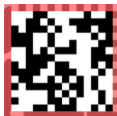
A data matrix showing finder pattern defects
