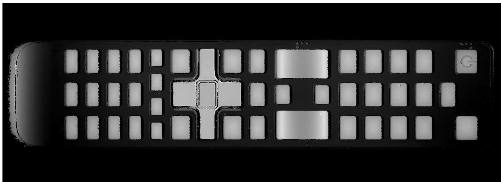
The ZMap with a reference plane previously calculated, an orientation to align the object and a reduced resolution
