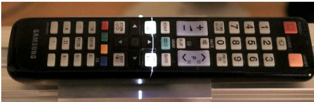
The remote controller on the laser triangulation acquisition setup
