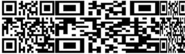
Square and rectangular QR codes (isotropy = 1, 0.5, and 0.5 from left to right)
