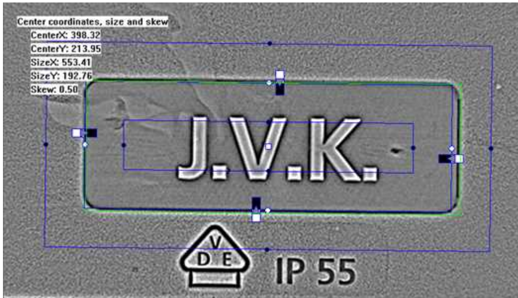
Rectangle measurement with EasyGauge on the mean curvatures
