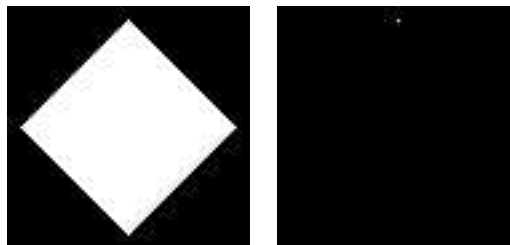
Source image (left) and top corner detected in the source image (white dot)
