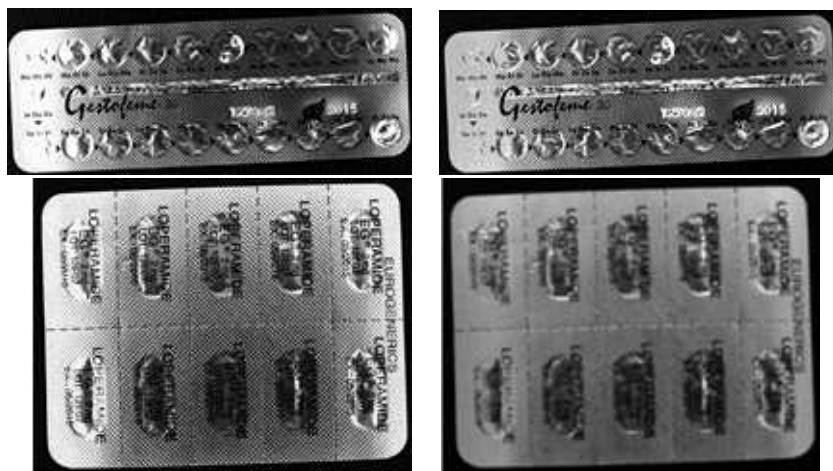
The albedos images: raw (left) and after correction with the flat images (right)
