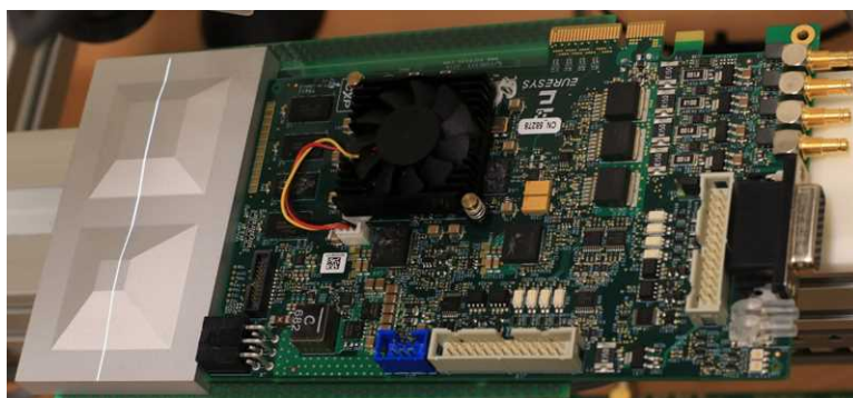
A PCB scanning setup with the associated calibration object
