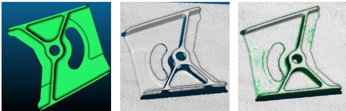
CAD model — sample point cloud — model and sample aligned (3D models courtesy of Direct Dimensions)
