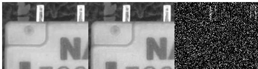
Comparing two noisy images for strict equality. Black pixels of the result image are non equal pixels.
