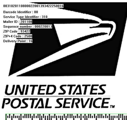
US Intelligent Mail bar code with highlighted position and decoded information
