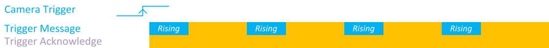
Trigger message transactions using default settings Case 1 and case 2: the camera acknowledges each message as expected Case 3: no acknowledgment from camera. Abort after 3 retries
