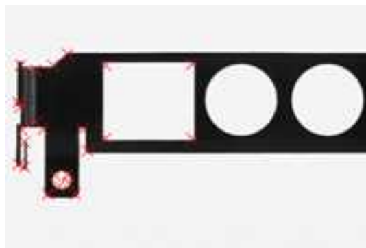
Corners are detected in the source image
